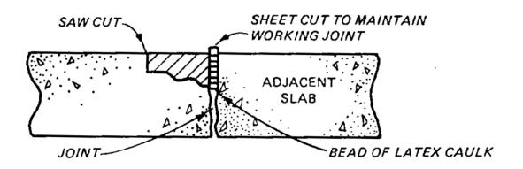
NOTE: USE COMPRESSIBLE SEPARATING MEDIUM WITH A MINIMUM THICKNESS OF 1/2" IN JOINT TO MAINTAIN AND PROTECT JOINT DURING PLACEMENT OF THE FRESH CONCRETE.
